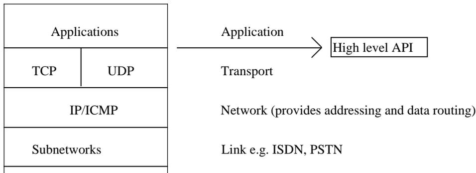
**Figure 2: TCP/IP model**
