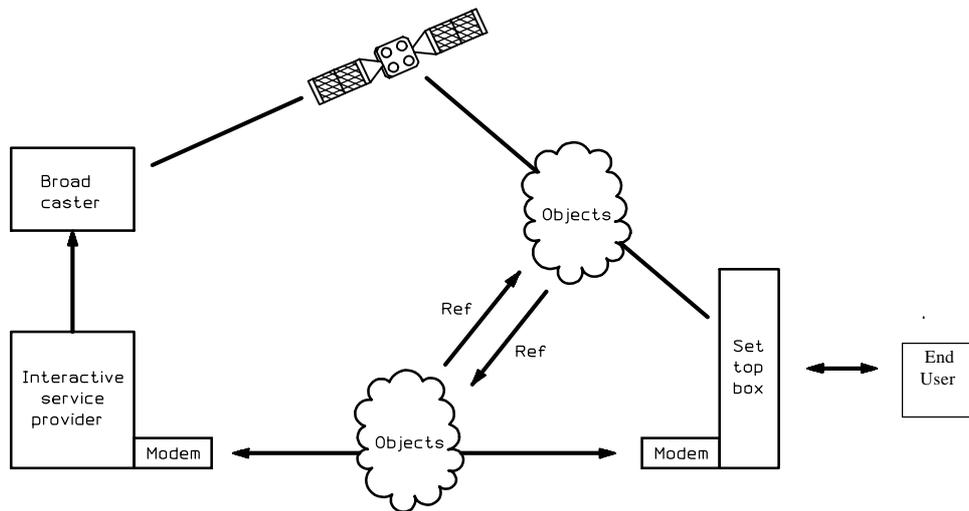
**Figure 1: High level system overview for Interactive Services (IS) supporting broadcast to the home with narrowband return channels**
