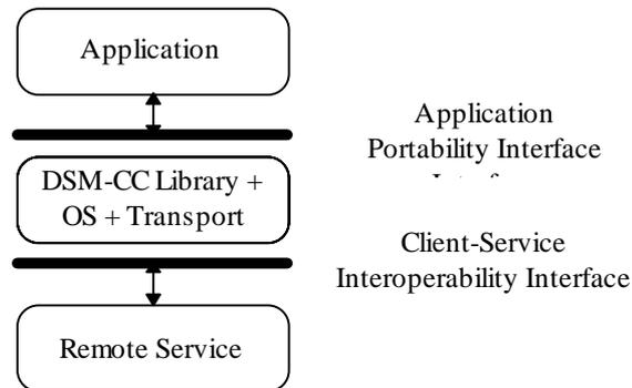
**Figure 7: Application and Service Interfaces**
