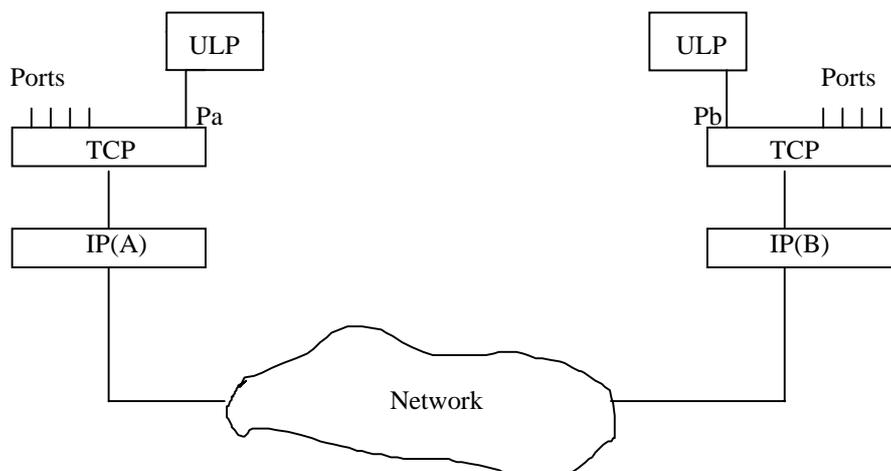
**Figure 4: TCP connection structure**
