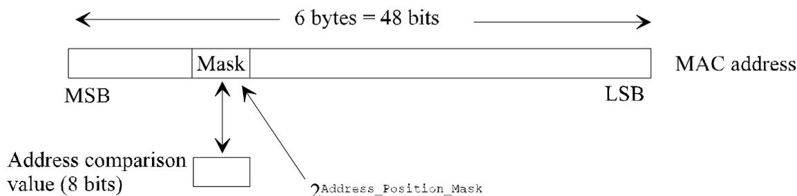
**Figure 29: Position of Mask in MAC address**
