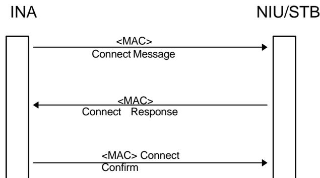
**Figure 30: Connection signalling**
