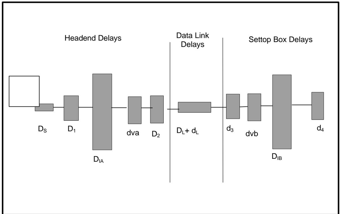
**Figure 22. System Model for Timing Analysis**
