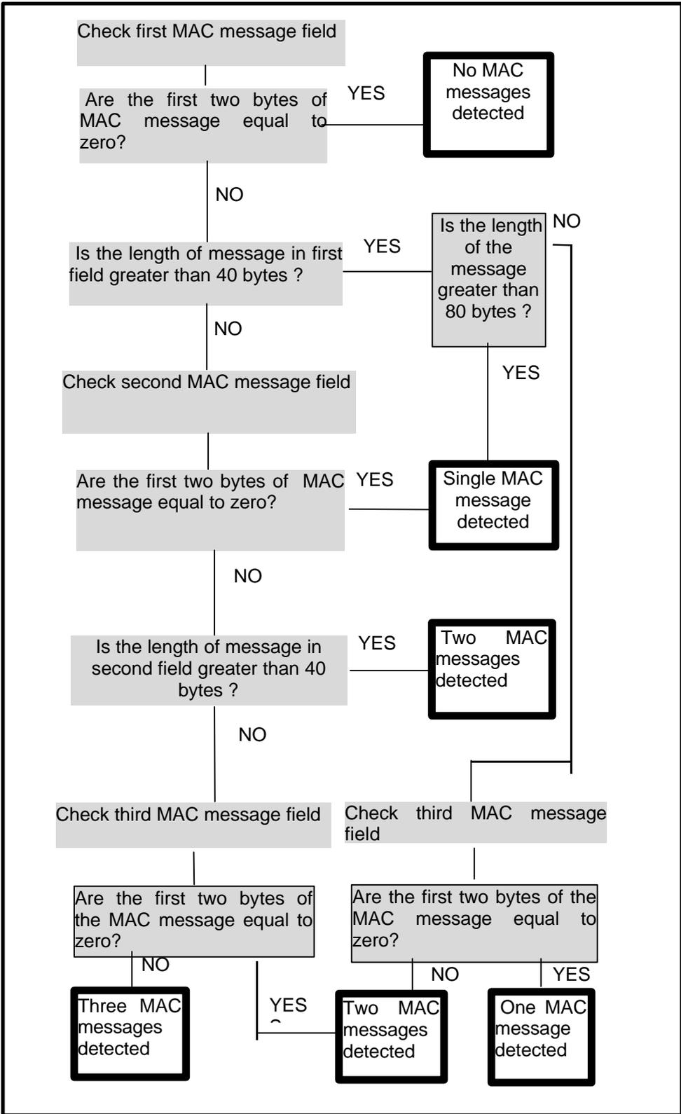
Figure 25 : Algorithm when MAC message are sent IB downstream
