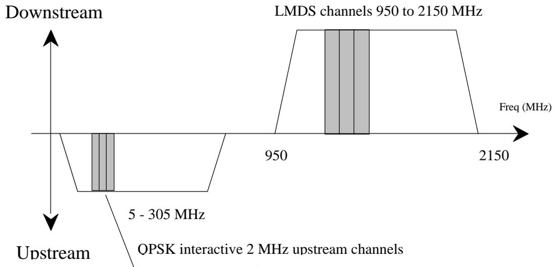
**Figure 3b : DVB preferred IF frequency ranges for LMDS interactive systems (IB)**
