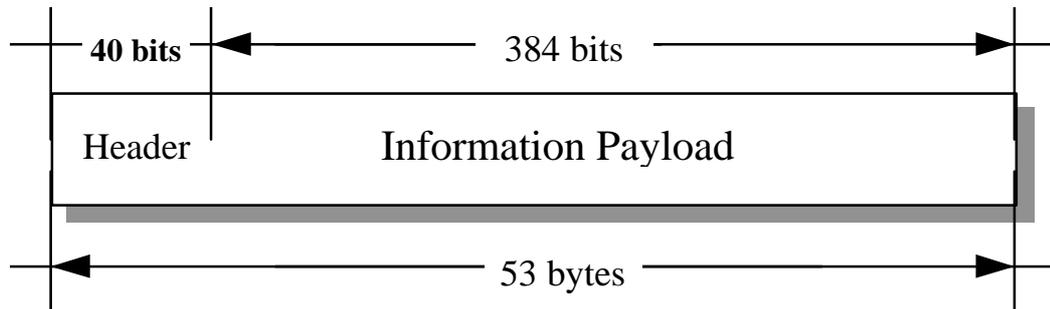
Figure 20: ATM cell format
