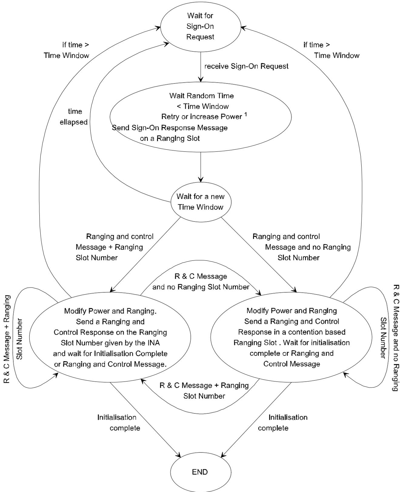
**Figure 28: State Diagram for Ranging and Calibration**
