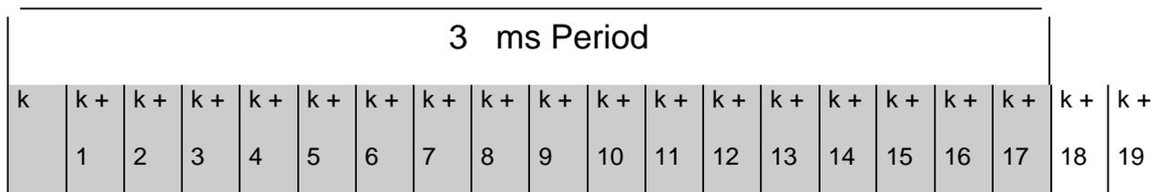
As the downstream and upstream bit rates are 3.088 Mb/s, there are 6 slot position references downstream during the transmission of 18 upstream packets. In the case of IB downstream, packet « k » is sent when the 3 ms time marker is received.
