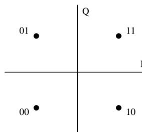
**Figure 8: Mapping for the QPSK constellation (downstream OOB)**
