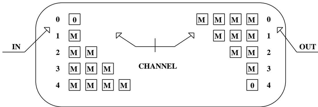
**Figure 19: Interleaver and De-interleaver structures**
