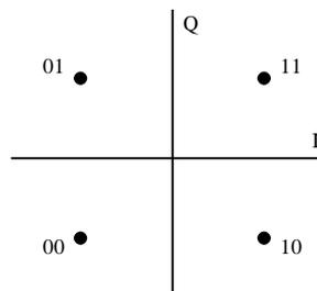
**Figure 7: Mapping for the QPSK constellation (downstream OOB)**
