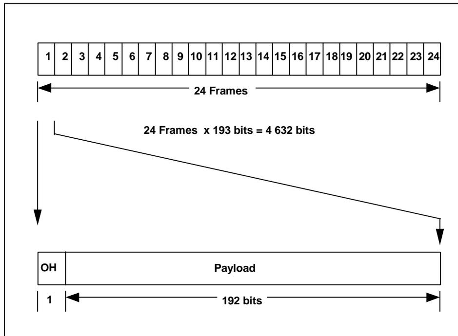
**Figure 17: SL-ESF Frame Structure**
