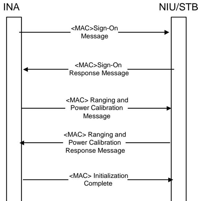
**Figure 30: Ranging and Calibration Signalling**
