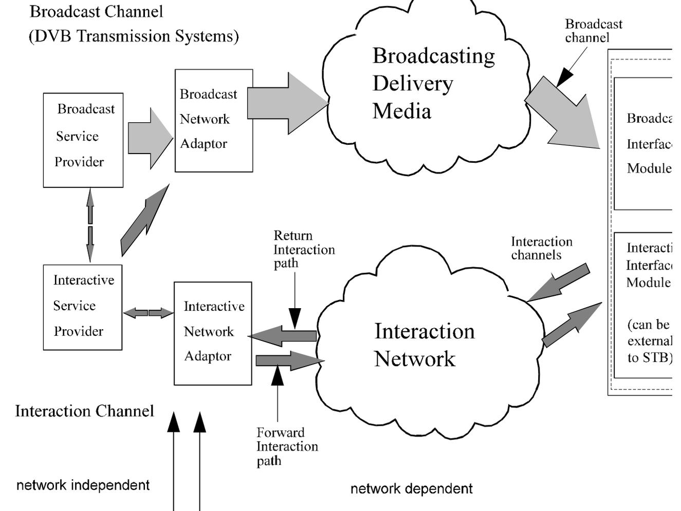
Figure 2a: A generic system Reference Model for Interactive System
