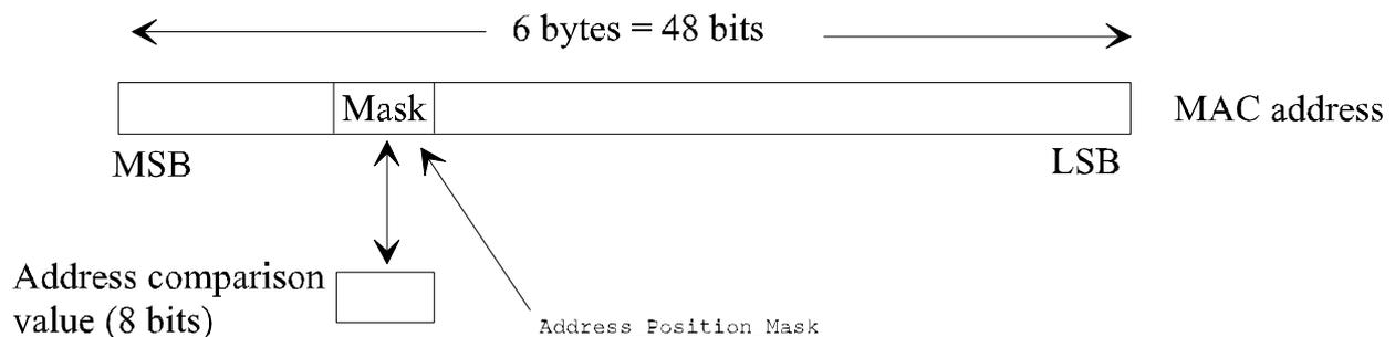
**Figure 31: Position of Mask in MAC address**
