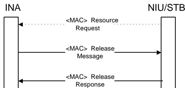
**Figure 34: Connection release signalling**
