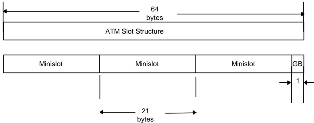
**Figure 36: Minislot Framing Structure**
