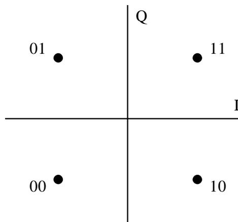
**Figure 12: Mapping for the QPSK constellation (upstream)**
