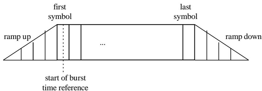
**Figure 15: Burst Ramp Up and Down**
