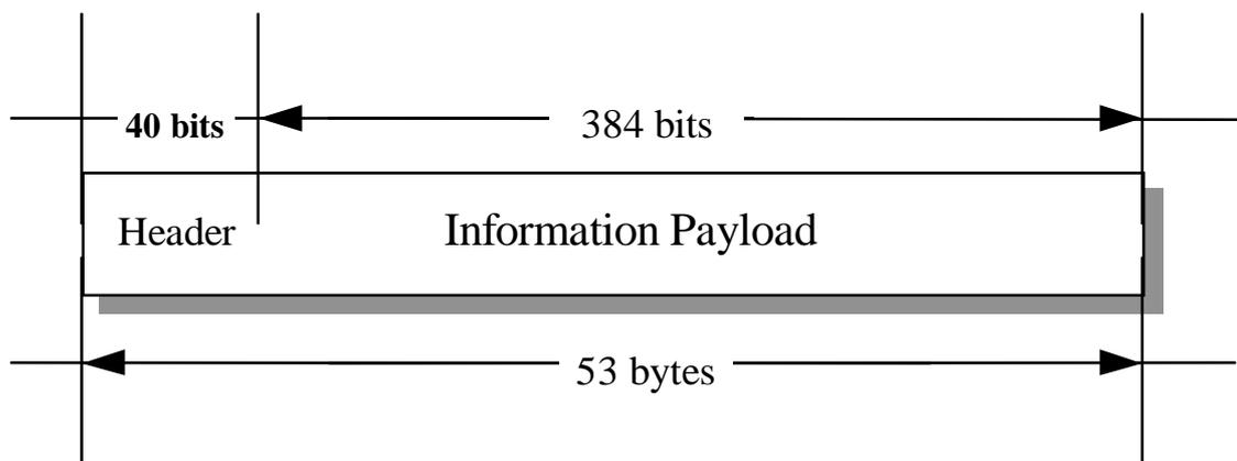
Figure 22: ATM cell format
