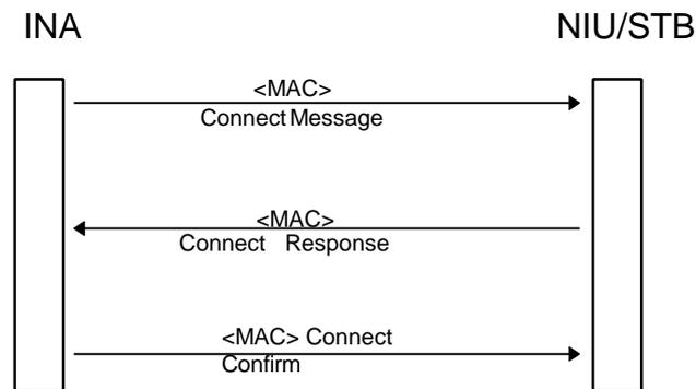
**Figure 32: Connection Signalling for the Initial Connection**
