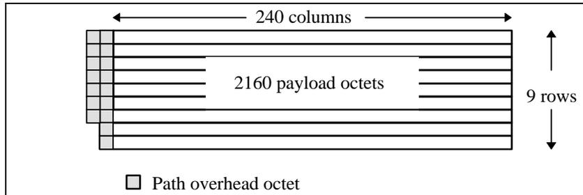
**Figure 21: Frame structure at 139 264 kbit/s**
