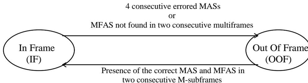
**Figure 20: Frame alignment state diagram**
