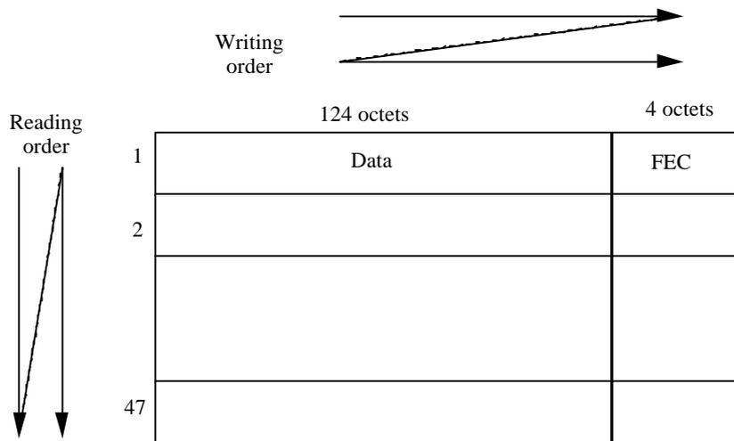
**Figure 4: Structure and format of the inter-leaver matrix**
