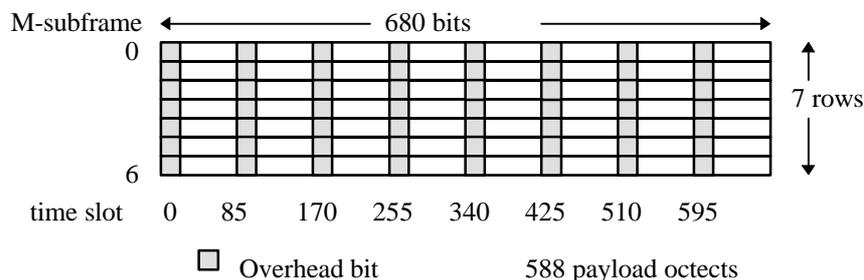
**Figure 19: Multiframe structure at 44 736 kbit/s**
