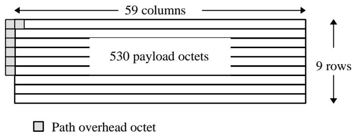
**Figure 16: Frame structure at 34 368 kbit/s**
