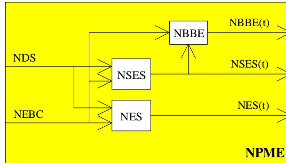
**Figure 25: Near-end Performance Monitoring Event (NPME) function**
