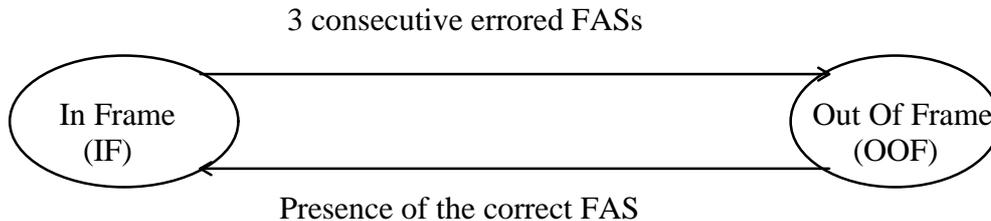
**Figure 9: Frame alignment state diagram**
