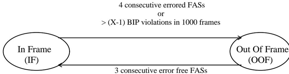
**Figure 23: Frame alignment state diagram**
