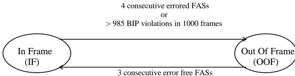
**Figure 18: Frame alignment state diagram**
