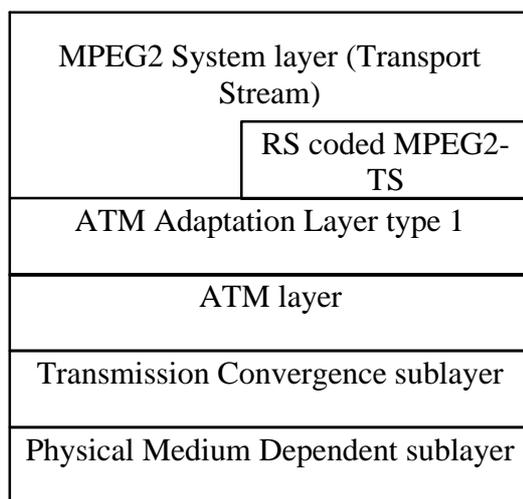
**Figure 2: Protocol stack for the adaptation process**
