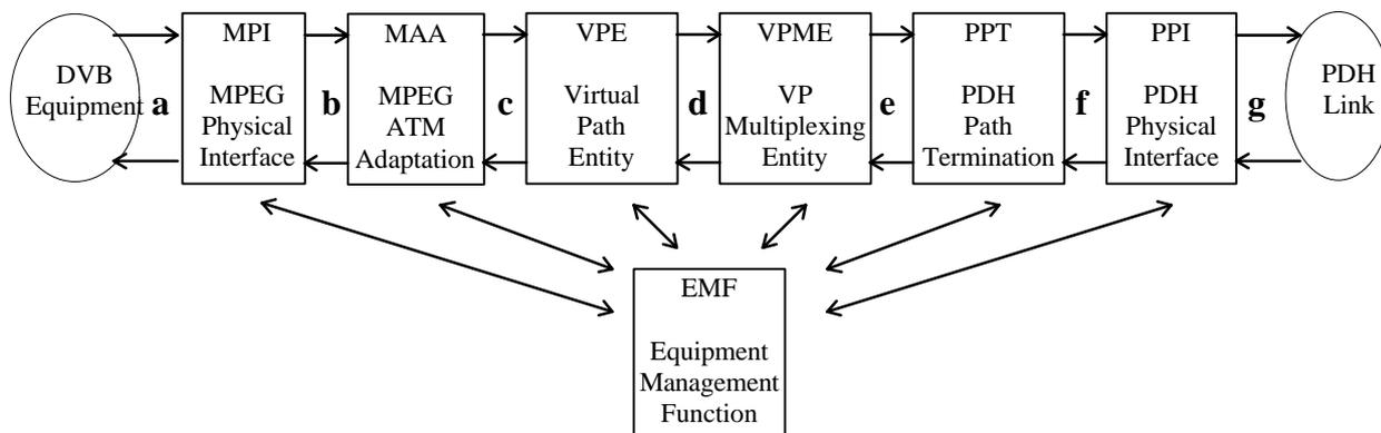
**Figure 1: Functional blocks of the Network Adapter**
