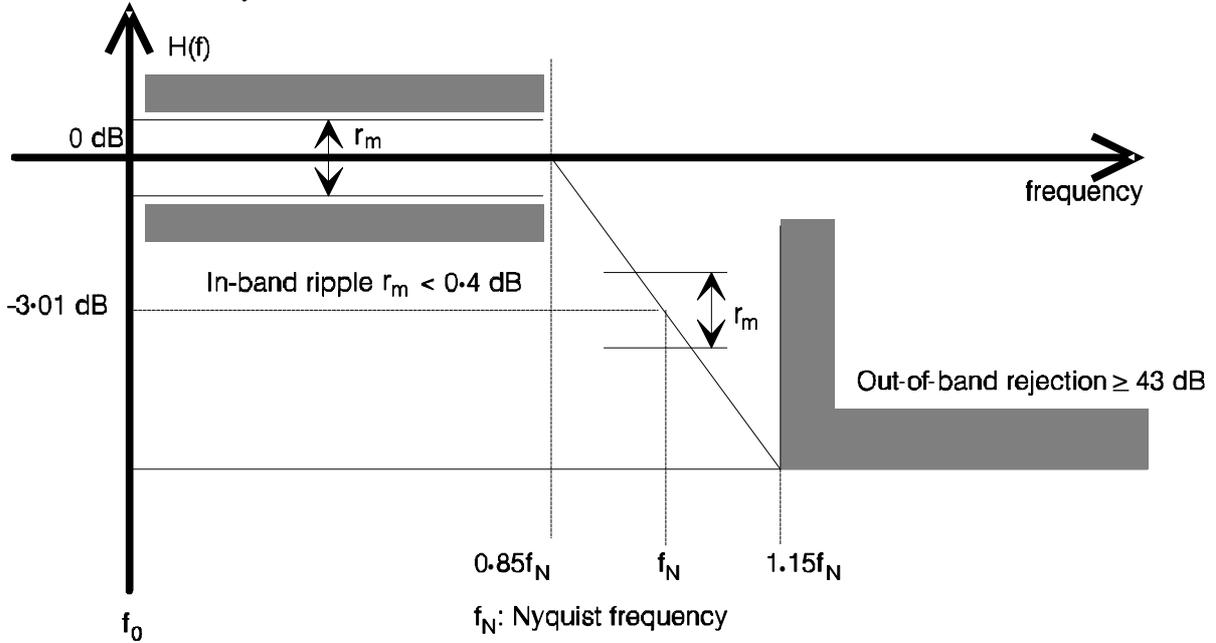
**Figure A.1 : Half-Nyquist baseband filter amplitude characteristics**
