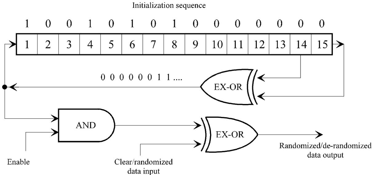
**Figure 3 : Scrambler/descrambler schematic diagram**
