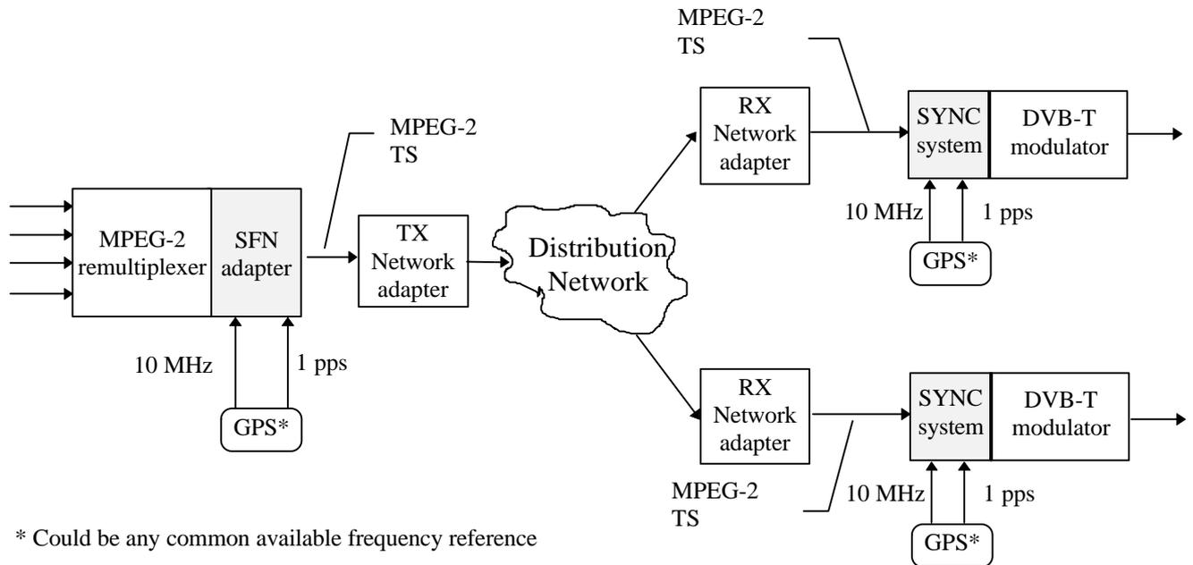
Figure 1. DVB-T primary distribution with SFN adaptation
