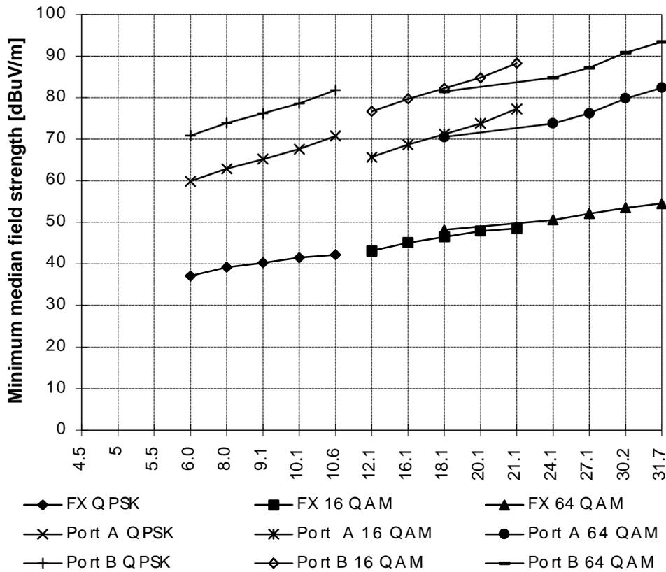
**Figure 6.6:** Minimum median field strength versus bit-rate for “good” coverage (95%), Band IV,  $T_g/T_u = 1/32$
