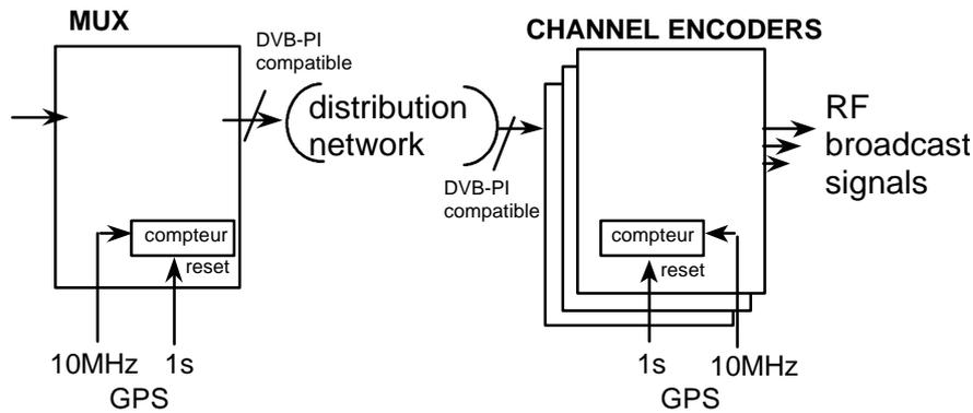
Figure 5.3 Mechanism for time reference
