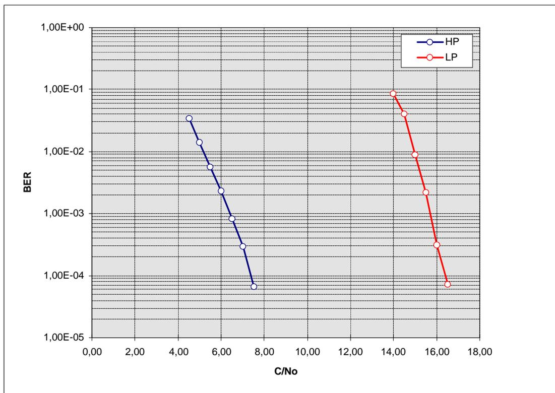
Figure 1.6: System performance for low and high priority bit-stream in a hierarchical transmission scenario
