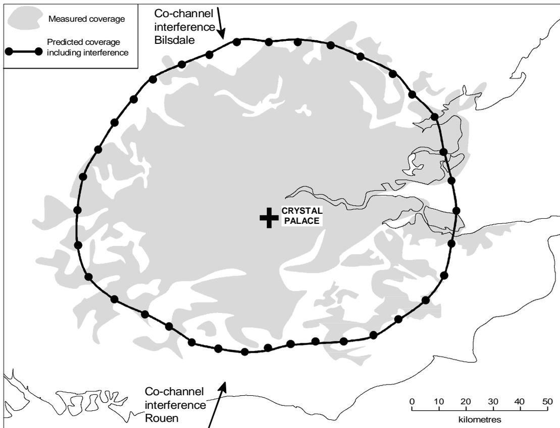
Fig. 6.9: Comparison of BBC measured and EBU computer generated test points/coverage for Crystal Palace analogue television on channel 33
