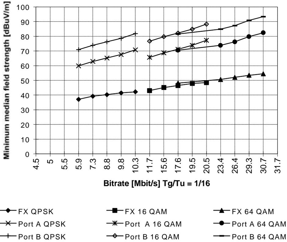
Figure 6.5: Minimum median field strength versus bit-rate for “good” coverage (95%), Band IV,  $T_g/T_u = 1/16$
