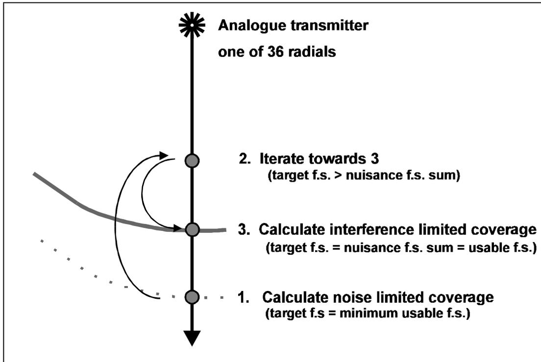
Fig. 6.7: Calculation of test points for the analogue interference limited coverage
