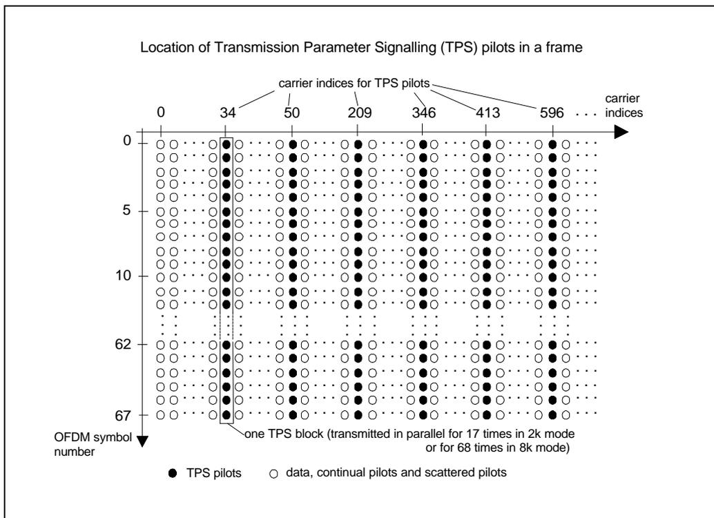
Figure 1.7: Location of TPS pilots in a frame containing data signals and pilots
