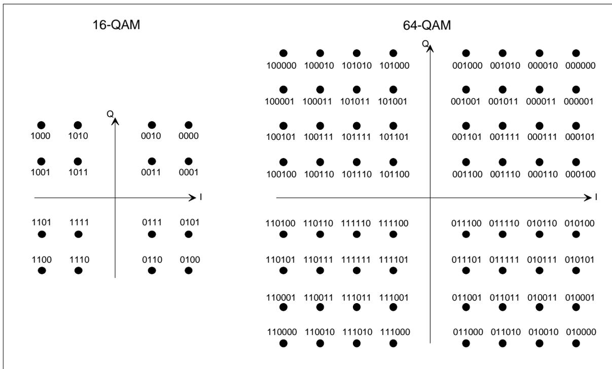
Figure 1.2: Constellation diagram for the hierarchical modulation ( $\alpha=2$ )
