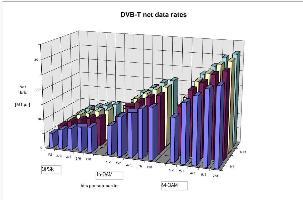
Figure 1.3: Net data rates in the DVB-T system
