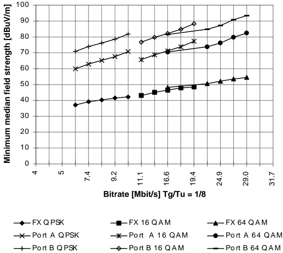
**Figure 6.4:** Minimum median field strength versus bit-rate for “good” coverage (95%), Band IV,  $T_g/T_u = 1/8$
