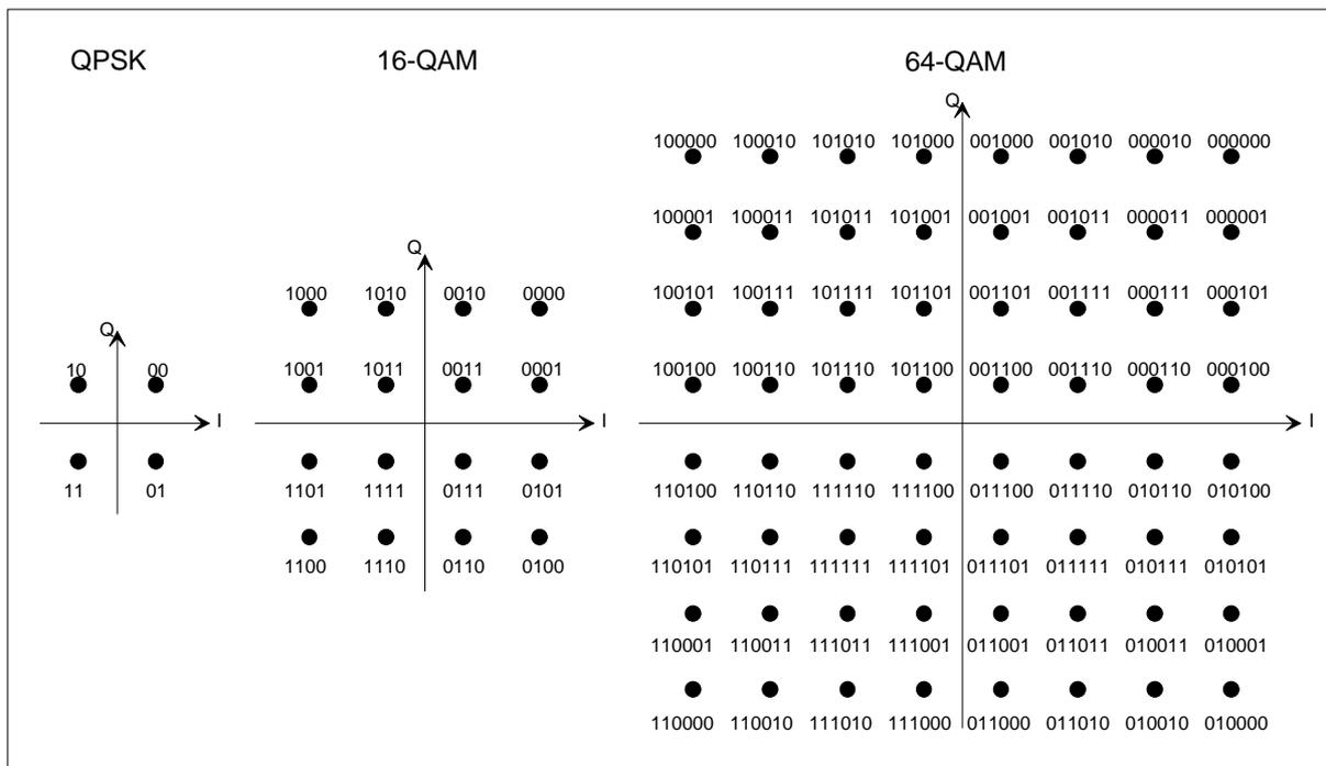
Figure 1.1: Constellation diagram for the modulation methods specified for DVB-T
