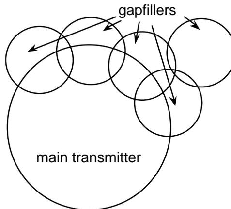
Figure 5.1 Gap-fillers fed from main transmitter
