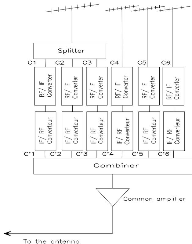
Figure 3.2 Typical structure of the multichannel repeater site
