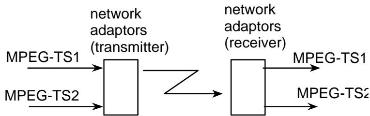
Figure 5.4 Distribution of 2 MPEG transport streams
