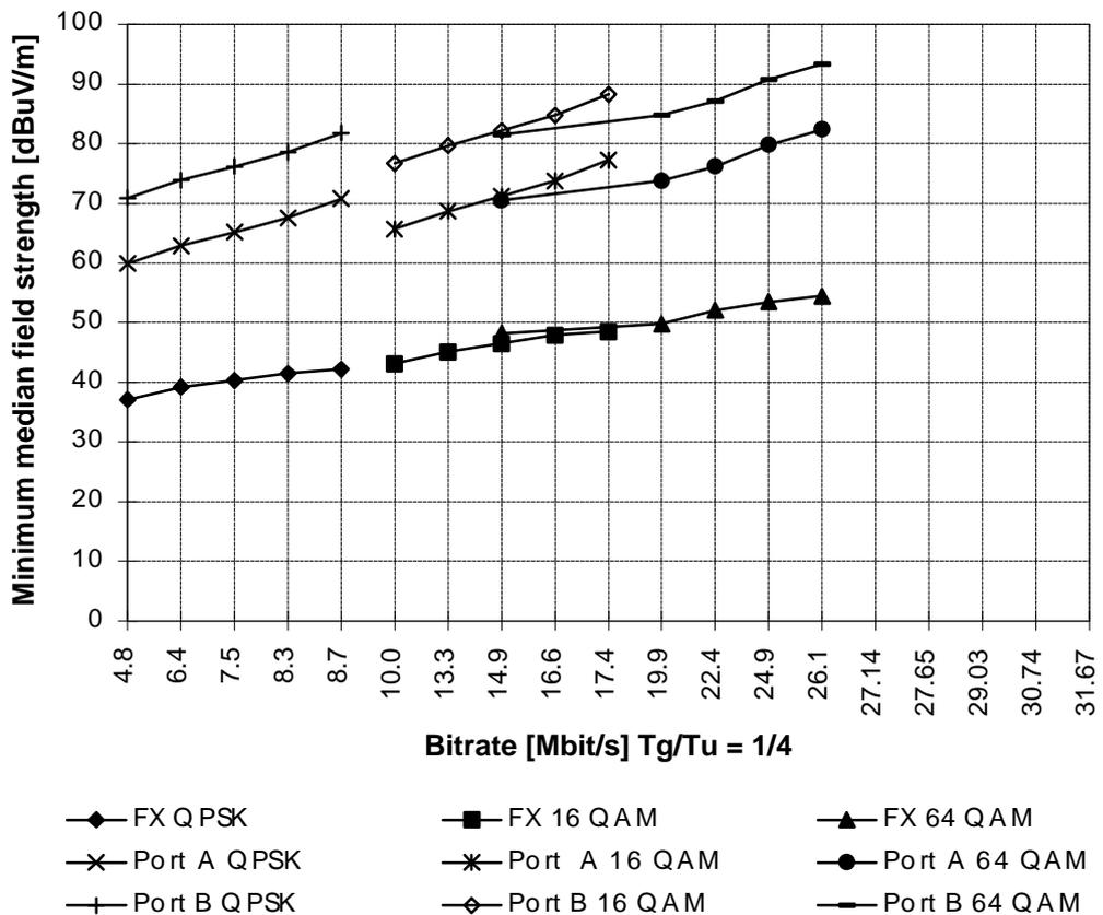
**Figure 6.3:** Minimum median field strength versus bit-rate for “good” coverage (95%), Band IV,  $T_g/T_u = 1/4$
