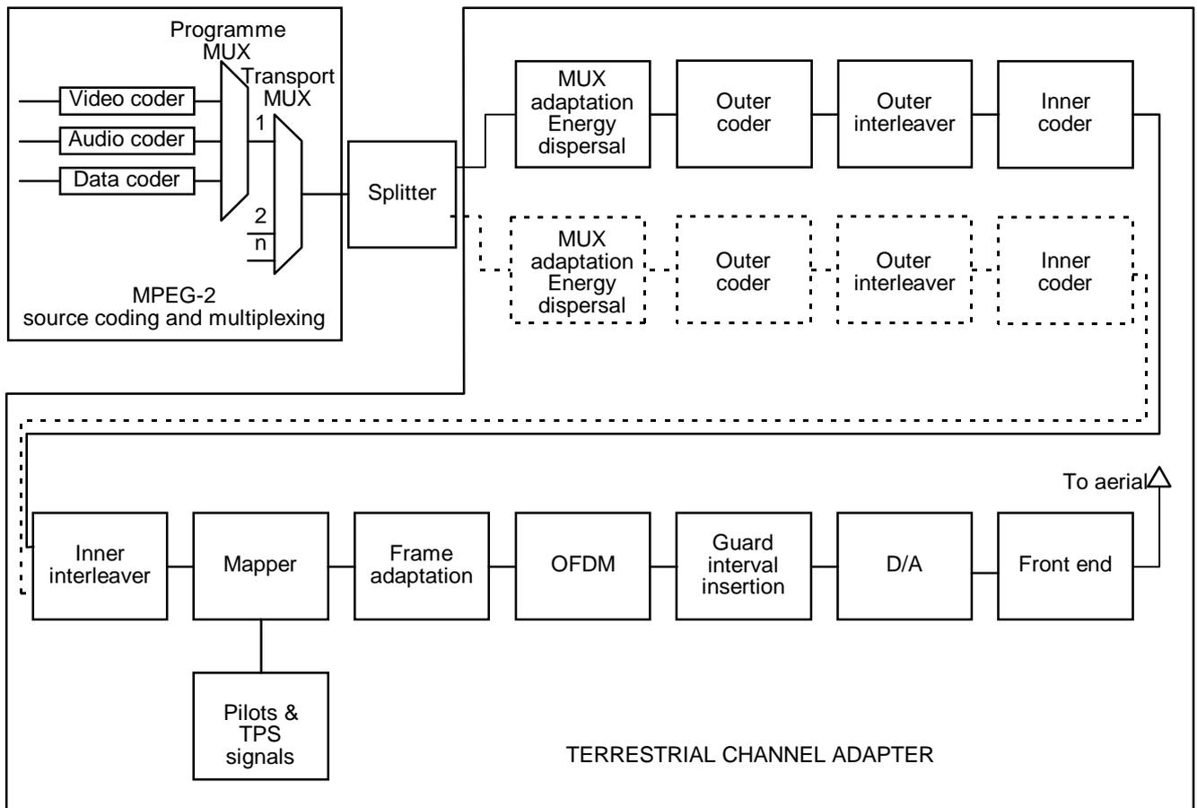
Figure 5: Functional block diagram of the system
