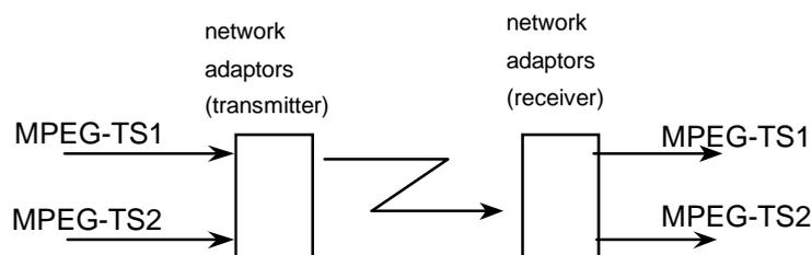
Figure 14: Distribution of 2 MPEG transport streams
