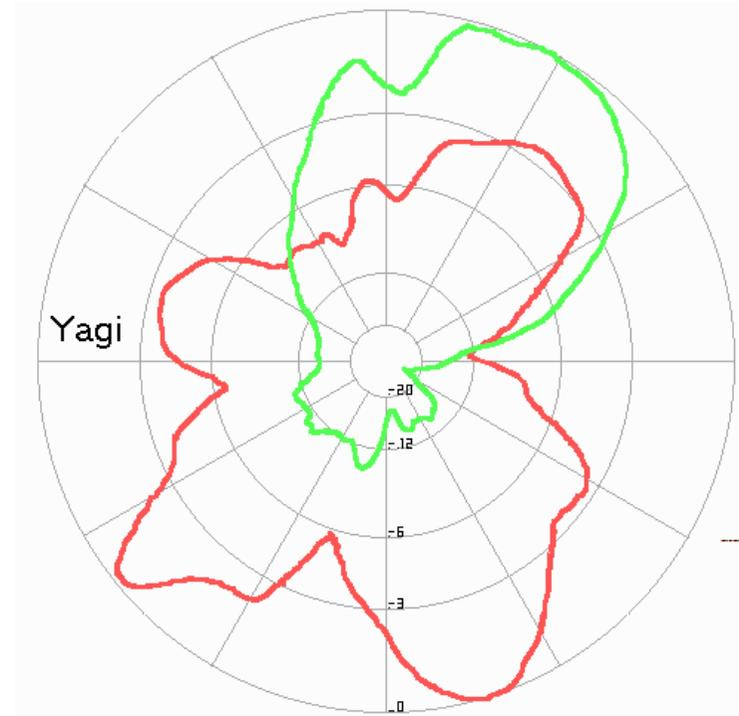
Examples of antenna patterns for two antenna types at an indoor location close to a wall, measured in The Netherlands, are shown in figure 15.
