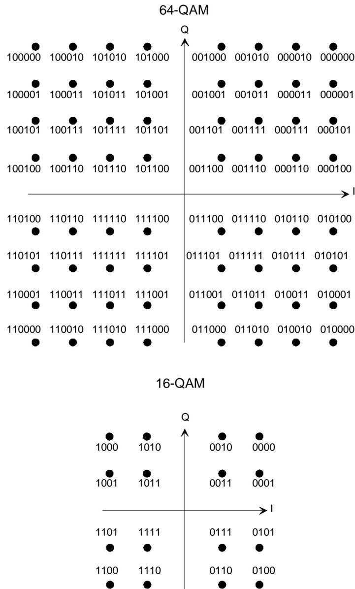
**Figure 2: Constellation diagram for the hierarchical modulation ( $\alpha=2$ )**
