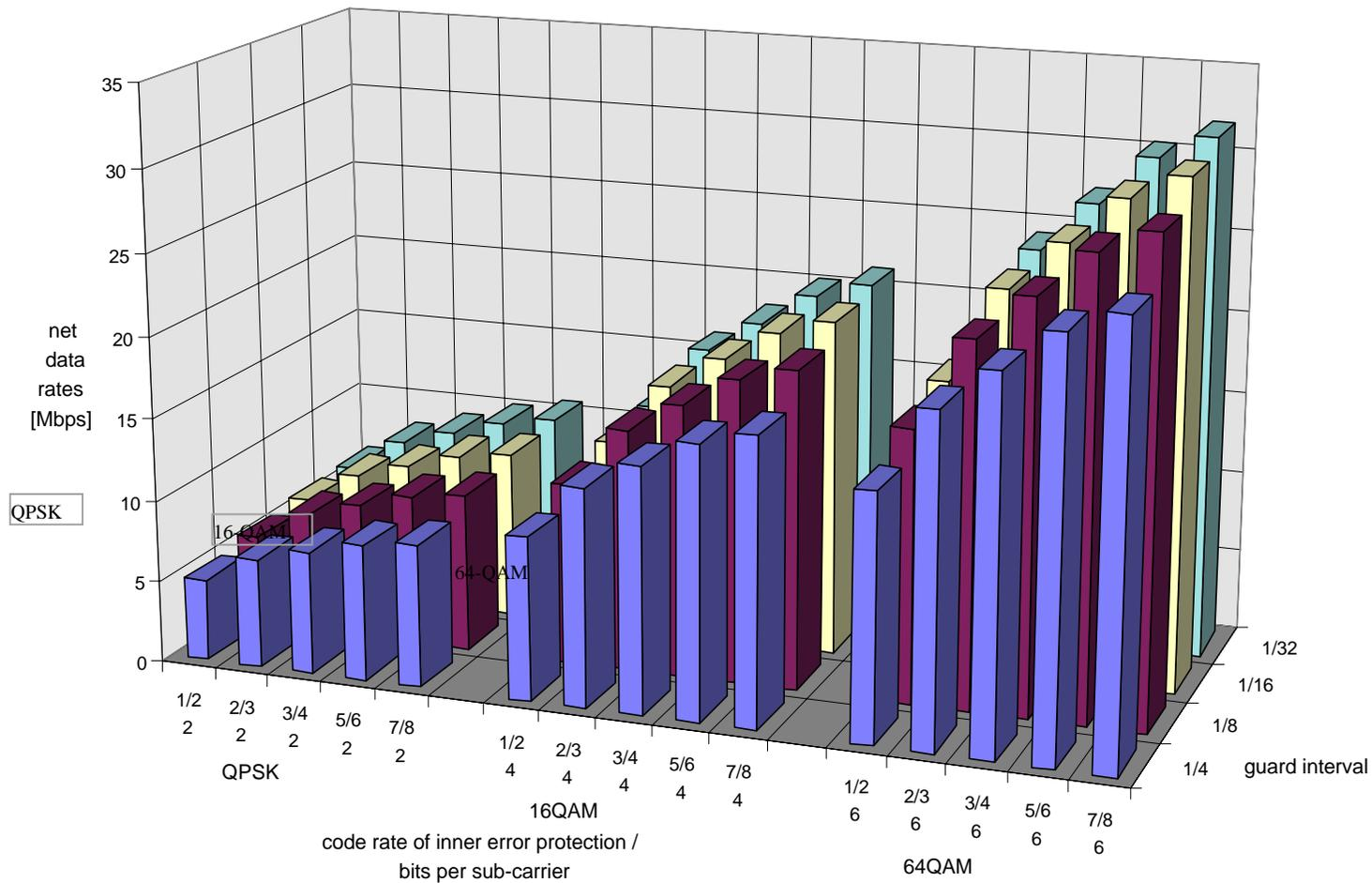
Figure 3: Net data rates in the DVB-T system
