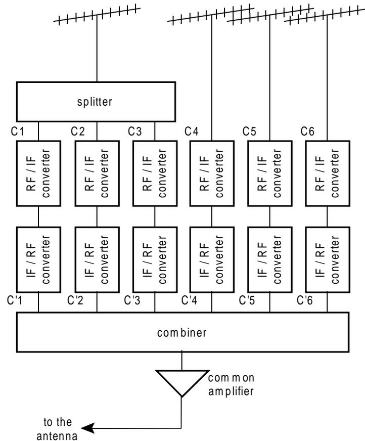
**Figure 10: Typical structure of the multi-channel repeater site**
