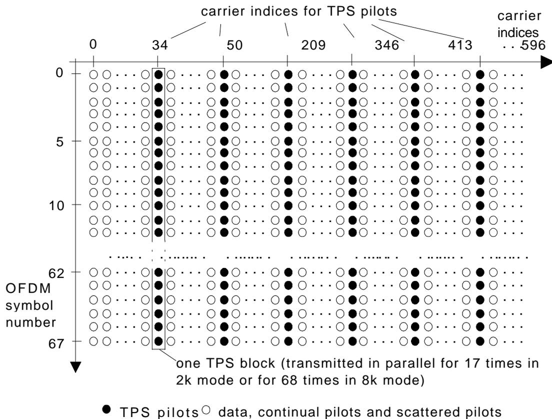
Figure 7: Location of TPS pilots in a frame containing data signals and pilots
