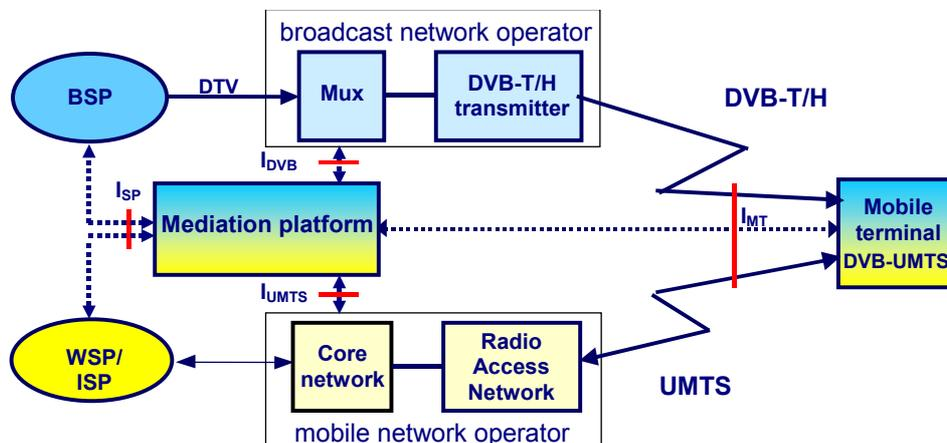
**Figure 1: Mediation platform concept and interface I<sub>MT</sub> in its context.**
