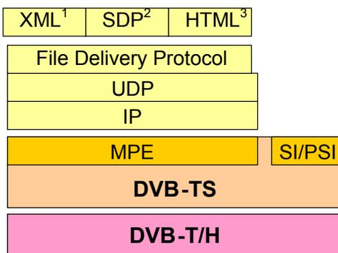
**Figure 5 Protocol stack architecture of the Service Discovery Channel** <sup>1,2,3</sup>.
